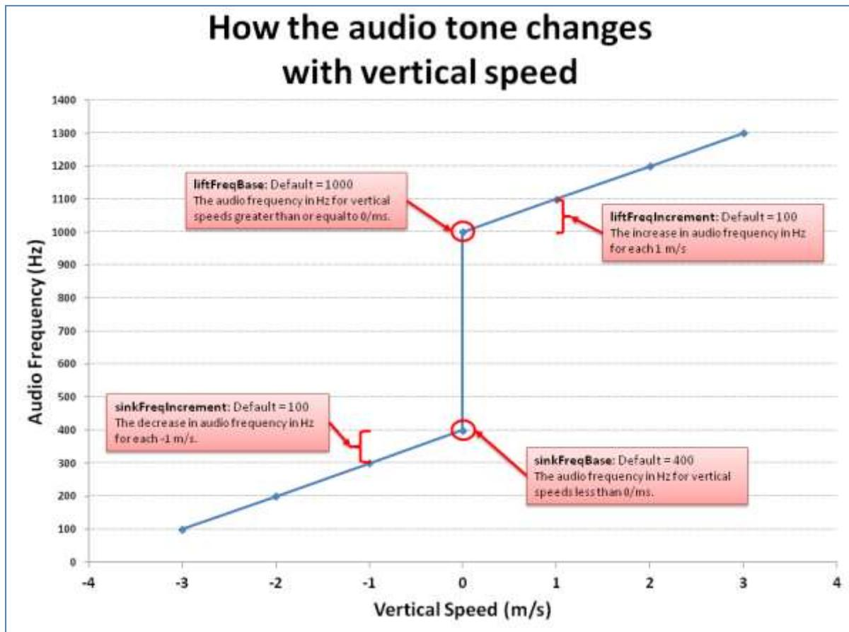
Note that in the most recent versions of the BlueFlyVario (from v7 onwards), the Audio Frequency cannot be played below 130Hz. If the combination of the settings and the measured vertical speed results in a calculated audio frequency below 130Hz the resulting sound will be clamped to 130Hz.
