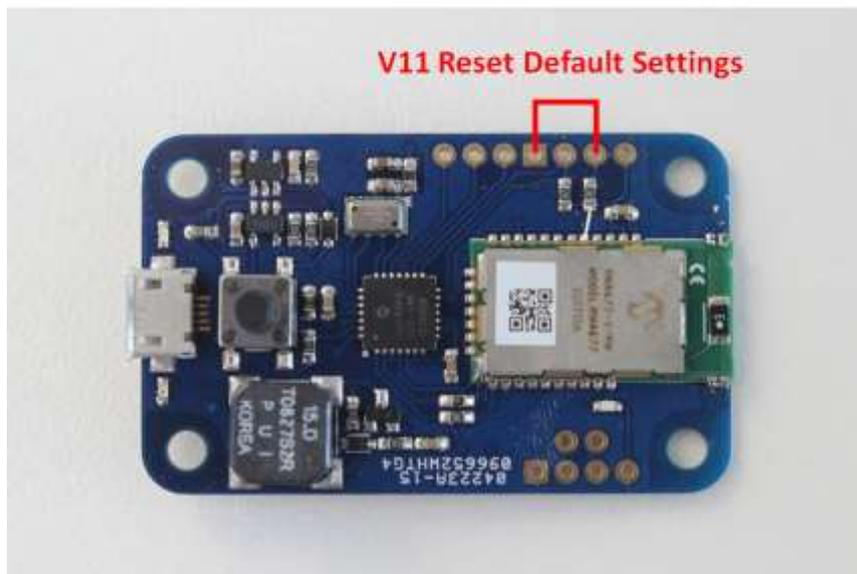
On v12 hardware you need to short SCL to Ground as well, but it is in a different spot.
