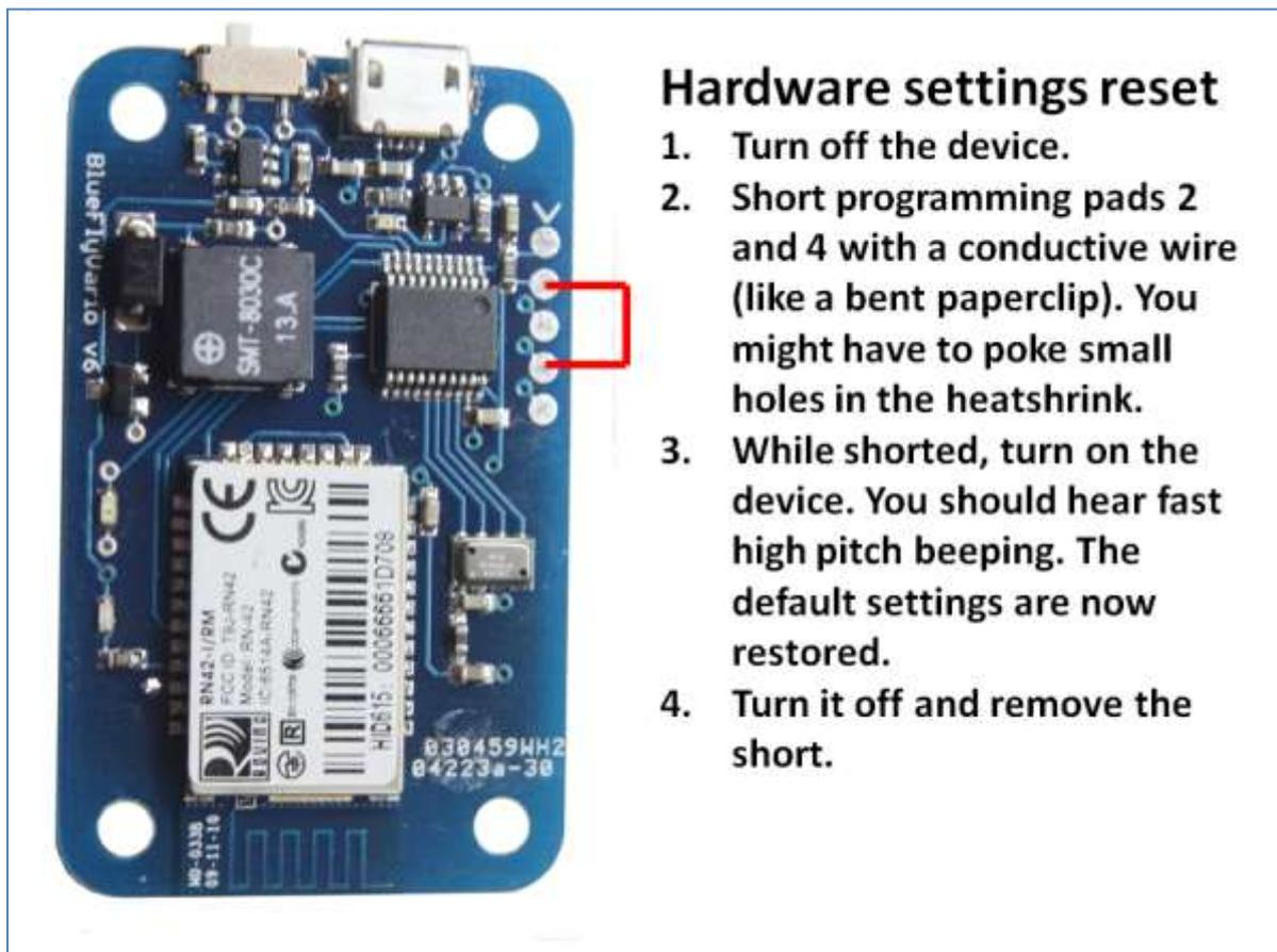
The procedure is similar for v11 and v12 hardware, but instead you need to short SCL to Ground.
