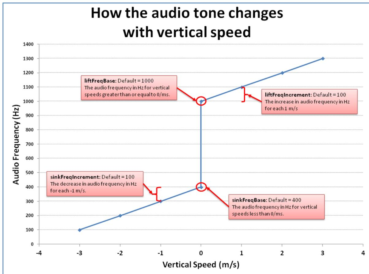
Note that in the most recent versions of the BlueFlyVario (from v7 onwards), the Audio Frequency cannot be played below 125Hz. If the combination of the settings and the measured vertical speed results in a calculated audio frequency below 125Hz the resulting sound will be clamped to 125Hz.
