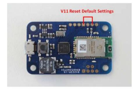
The procedure is similar for v11 and v12 hardware, but instead you need to short SCL to Ground.
